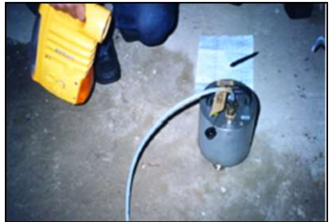
Fig. 4 Ambient vibration record from the traffic load with seismometer on ground level
