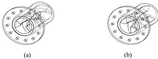
Fig. 2. Swirling nozzles; (a) 30 Degree Swirling Nozzle, (b) 60 Degree Swirling Nozzle
