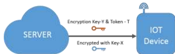
Fig.3 Server providing token and new encryption key
