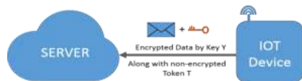
Fig.4. Device will send encrypted data and token for further communication
