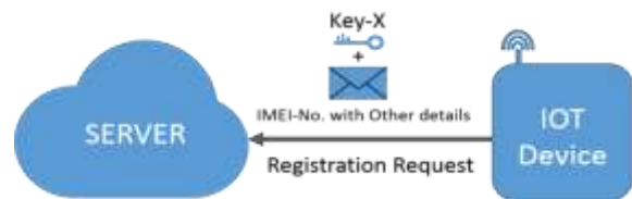
Fig.2. Device registration request encrypted with Key-X
