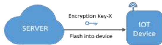
Fig.1. Server providing key-X to device, flash using flasher.
