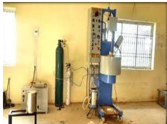
Fig 4: A stir casting setup as shown in Figure, consist of a Coke fired Furnace and a stirrer assembly.
