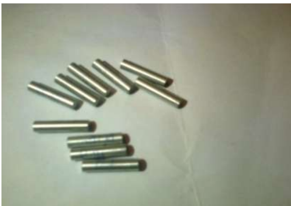
Fig 6: Wear test specimens
