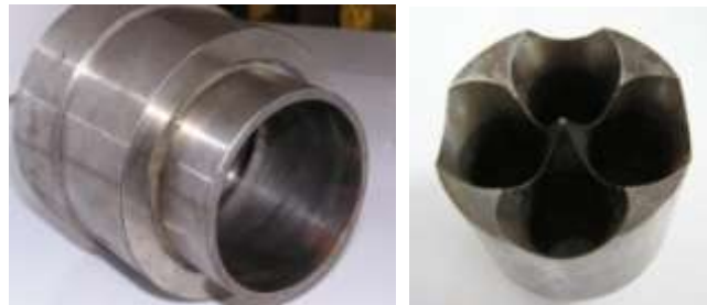
Fig. 7 Briquetting press nozzle (left), pelleting insert with four holes (right) [14]
