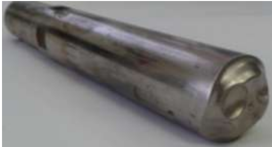
Fig. 1 Pressing piston as a tool of briquetting press
