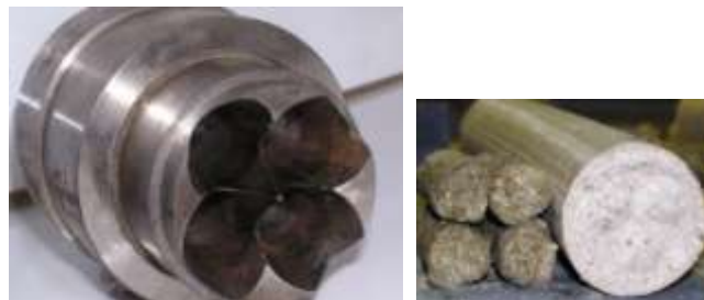
Fig. 8 Pelleting insert installed within the briquette nozzle (left), comparison of extrusion – pellets/briquette (right) [14]
