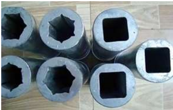
Fig. 4 Basic parts of the pressing chamber
