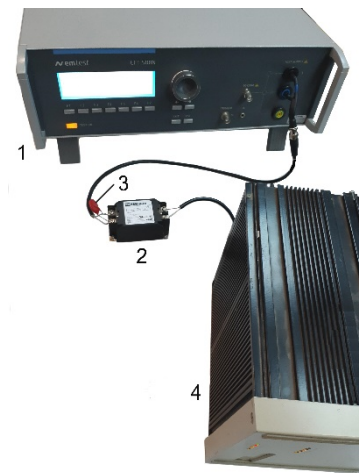
Fig. 6. Testing EFT resistance of a DPR fitted with 316NN63 power supply and external NBM-06-471 filter connected in series. 1 – EFT generator (EFT500N8); 2 – NBM-06-471 filter; 3 – varistor; 4 – REC316 type (ABB) DPR.
