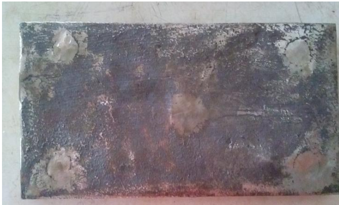
Figure 5. FCD 40 Sand Casting Workpiece
