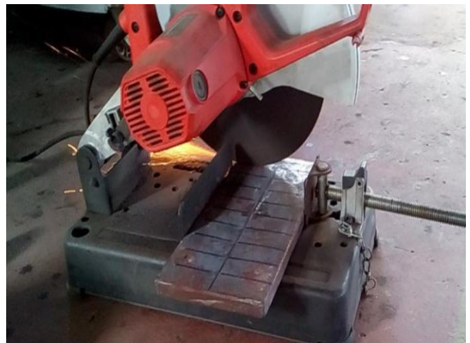
Figure 7. Initial Cutting of the Workpiece
