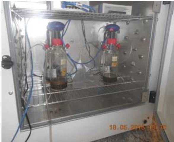
Figure 1: The digester system and some of its components.
