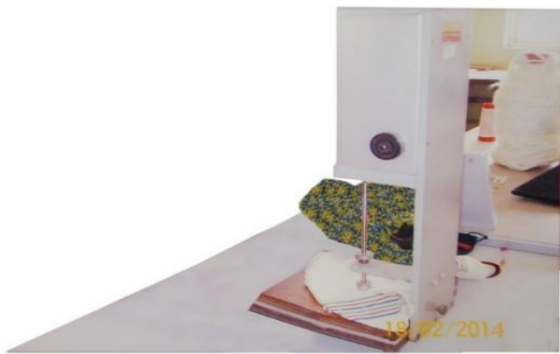
Figure 3: Testing Fabric Thickness using Essdiel Thickness Gauge
