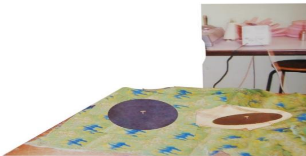
Figure 6: The Application of Drape Meter on both Akwete Fabric and Nigeria Cotton Wax Fabrics.
