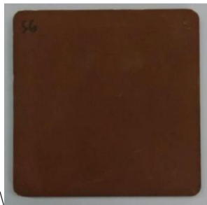
Figure 8. Body homogeneous ceramic Floor with the use of 10% tailings
