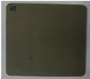
Figure 7. Body ceramic Floor with the use of 62.5% tailings
