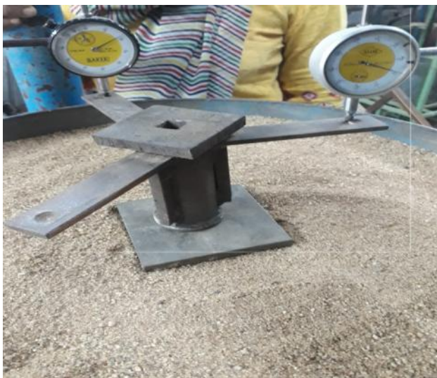
Figure 5: Model Test setup for plain raft foundation
