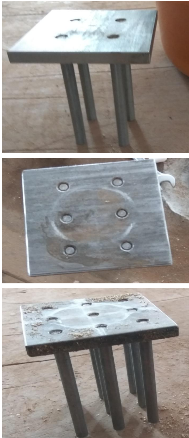
Figure 3: Fixing of piles and raft according to the test requirement
