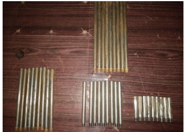
Figure 4: Model Steel Piles.
