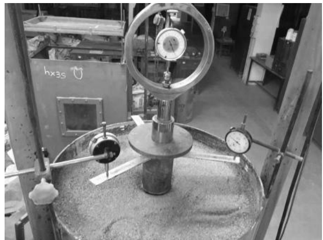
Figure 5: Model test set up with connector, proving ring and dial gauges
