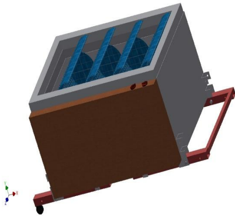
Figure 2c: AutoCAD of the maize roaster with legs collapsed
