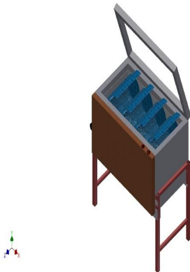
Figure 2d: AutoCAD of the maize roaster with legs unfolded
