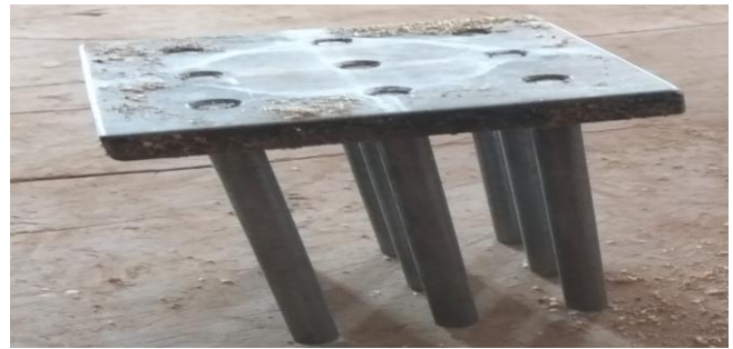
Figure 7: Raft with 9 piles arrangement
