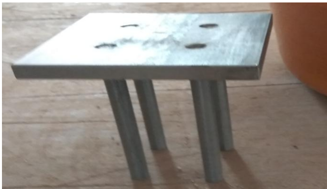
Figure 5: Raft with 4 piles arrangement
