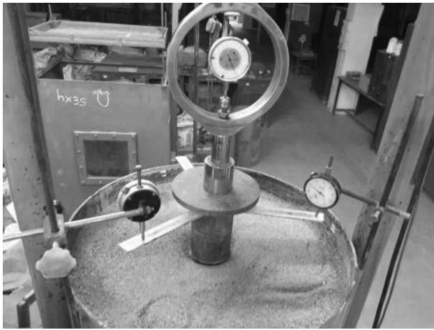
Figure 8: Model Test setup for plain raft foundation
