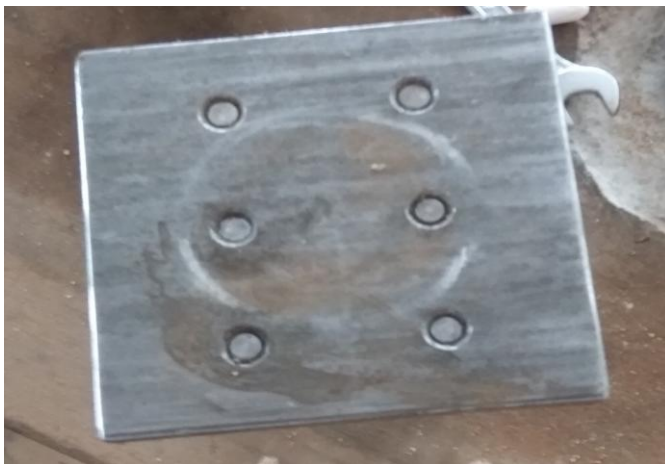
Figure 6: Raft with 6 piles arrangement
