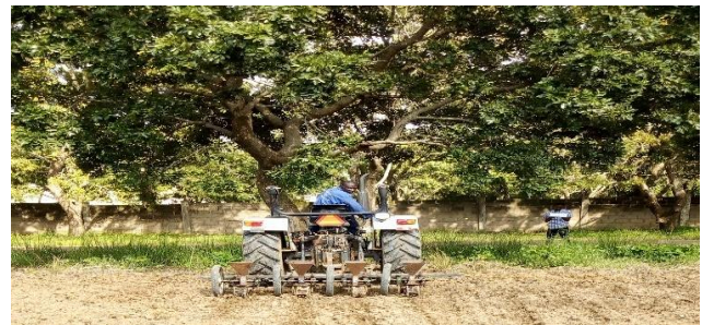
Figure 1 Developed Soybean Planter mounted on the tractor planting on the field.
