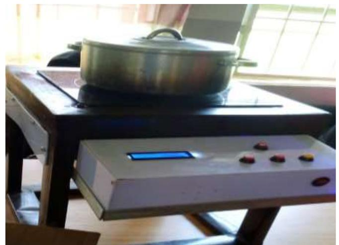
Figure 10: Testing of 24V Solar Powered DC induction Cooker
