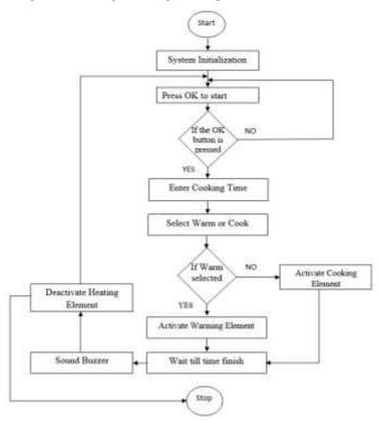
Figure 2: Flow Chart of the Sequence of operation of the Solar Powered DC Induction Cooker
