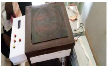
Figure 8: Pictorial View of Solar Powered DC induction Cooker
