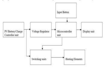
Figure 1: Block diagram of adigital solar-powered DC induction cooker
