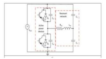
Figure 4: IGBT switching arrangement
