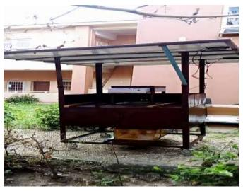
Figure 9: Assemblage of 24V Solar Powered DC induction Cooker
