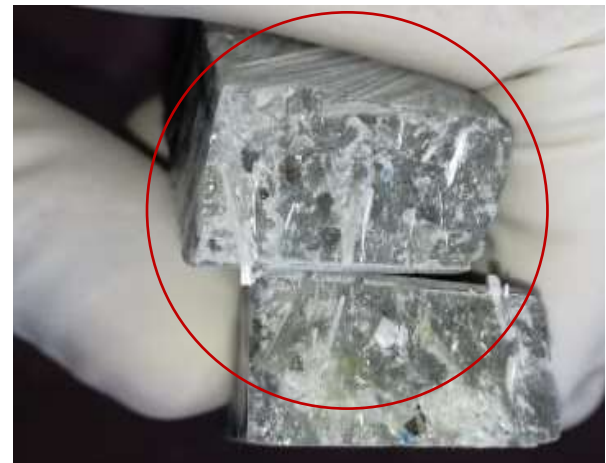
Fig. 6 Fracture Behavior of the Specimen Prepared Employing 35%–65% Recyclate and Resin Contents by Weight
