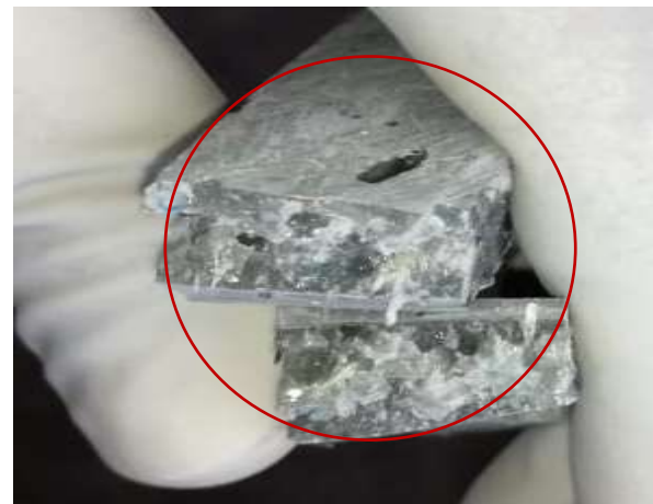
Fig. 7 Fracture Behavior of the Specimen Prepared Employing 40%–60% Recyclate and Resin Contents by Weight
