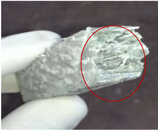
Fig. 8 Fracture Behavior of the Specimen Prepared Employing 50%–50% Recyclate and Resin Contents by Weight
