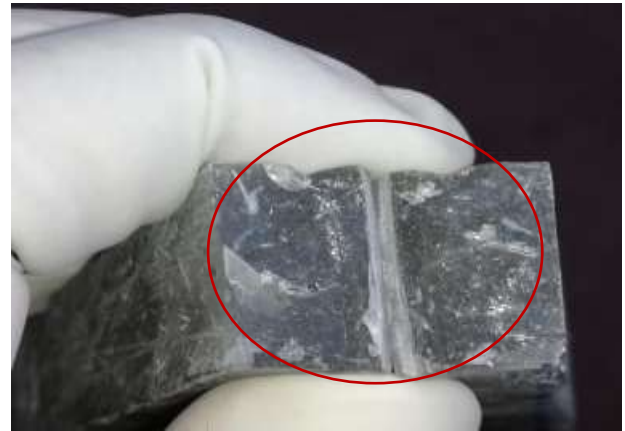
Fig. 5 Fracture Behavior of the Specimen Prepared Employing 20%–80% Recyclate and Resin Contents by Weight
