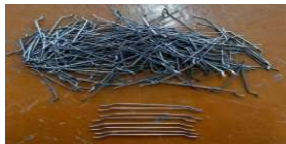
Figure 7 End Hook Steel Fibre. (Actual Photo inConcrete Lab.).
