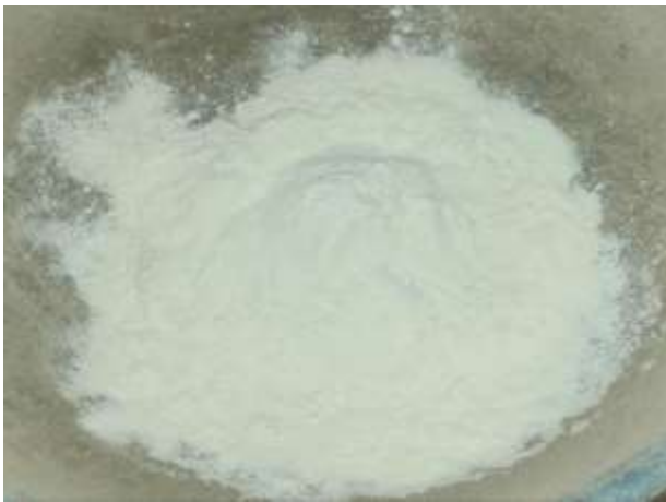
Figure 12 Pure Fine 99.99 % Silica Fume. (Actual Photo in Lab).
