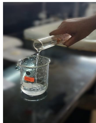
Figure 12. Addition of Sphatika Solution to the Guar gum mixture
