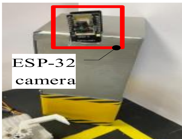
Fig. 10. Passive surveillance system using ESP-32 camera.
