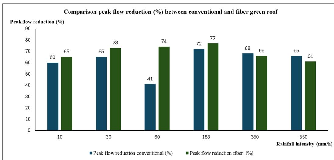
Fig 7 Graph of peak flow reduction (%) comparison between conventional and fiber green roofs.
