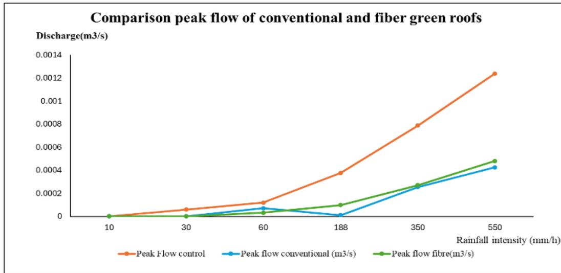
Fig 6 Graph of peak flow (m<sup>3</sup>/s) comparison between conventional and fiber green roofs.
