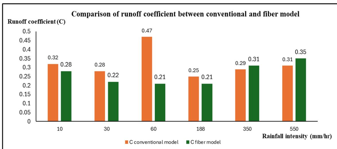
Fig 9 Graph of comparison of runoff coefficients between conventional and fiber models.
