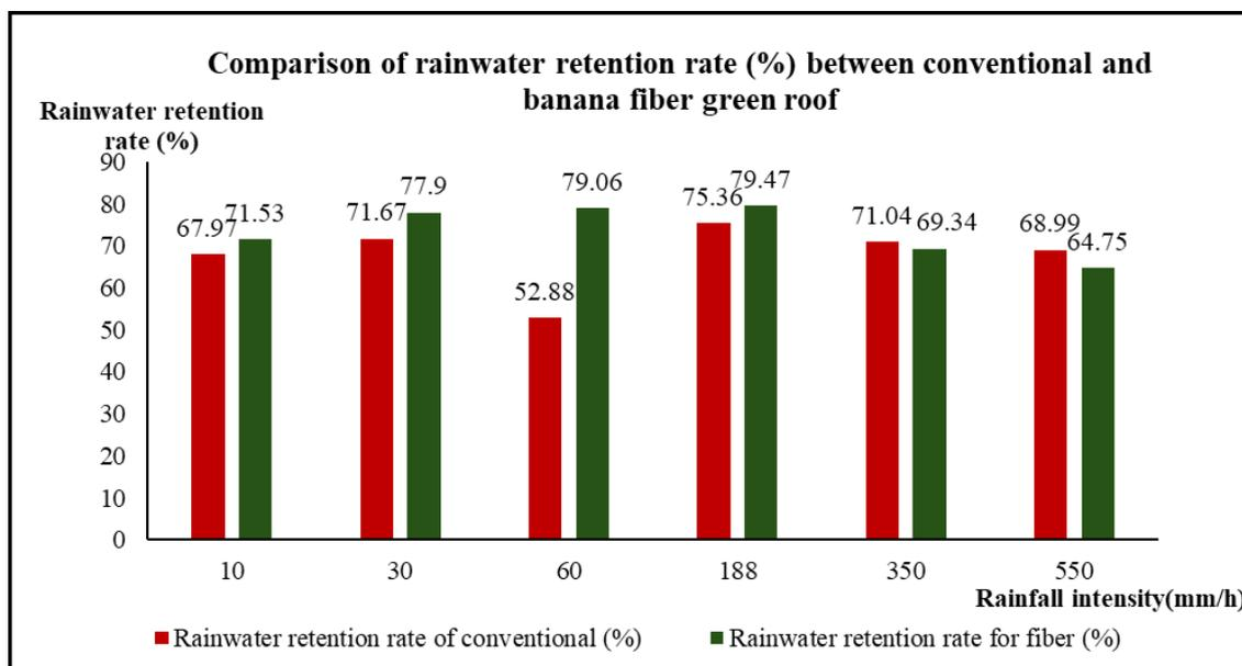
Fig 8 Graph of rainwater retention rate (%) comparison between conventional and banana fiber green roofs.
