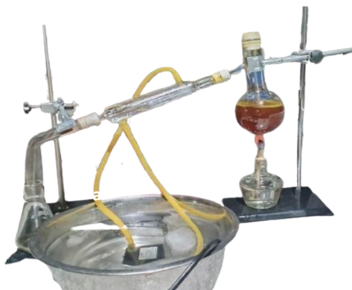
Figure 2. Improved steam distillation setup with a flask-distiller (a), condenser (b), receiver-flask (c), heat source-alcohol lamp (d), and distilled water (e); the dried flowers were loaded into the distiller with heat vaporizing the volatile oil through a condenser cooling into liquid, then the product was separated through a separator funnel.
