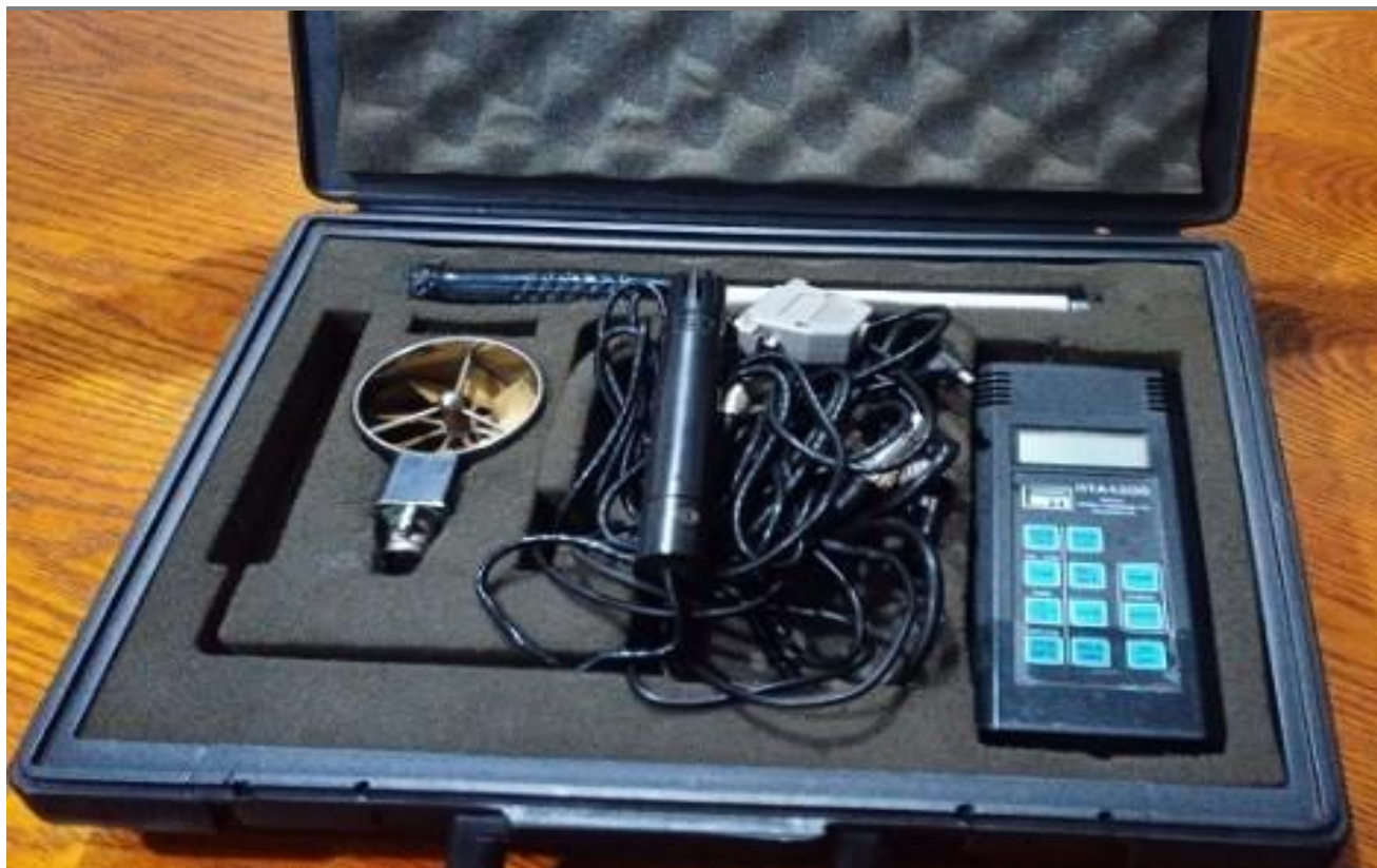
Fig 3. Tachometer used to measure the air flow rate over the fluidized bed
