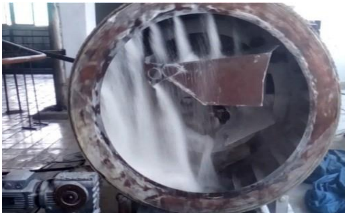
Fig 4. Particle film in rotating drum
