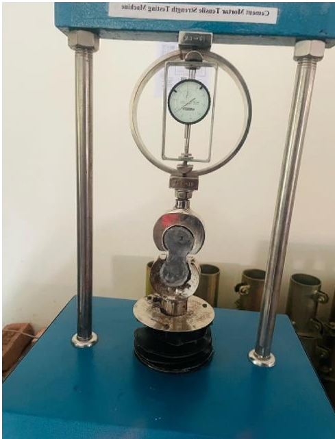
Figure 2.7: Tensile Testing Machine Used in Order to Test the Tensile Strength of the Block
