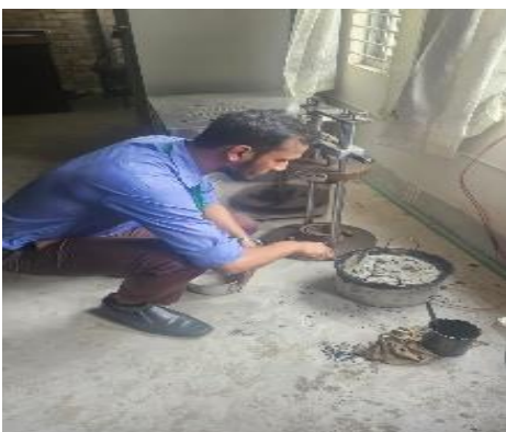
Figure 8: Mixing of CA, FA and Filler respectively and heating them on Electric Stove
