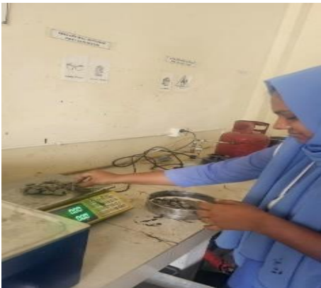
Figure 6: Weighting of CA, FA and Fillers according to their amount required with respect to Bitumen Percentages.
