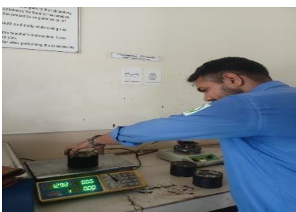
Figure 12: Taking SSD Weight after 30 minutes of water bath at 60 0 C
