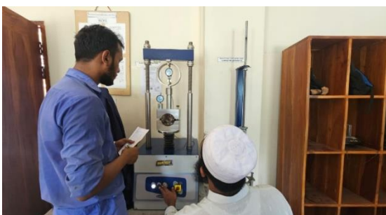
Figure 13: Putting the Specimen inside Marshall Testing Machine to obtain values
