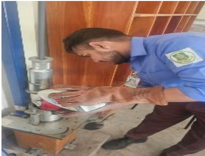
Figure 10: Adding the bituminous mix into the compaction machine and compacting to make a specimen.
