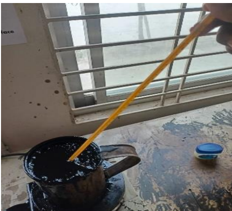
Figure 7: Heating of Bitumen till its melting point.
