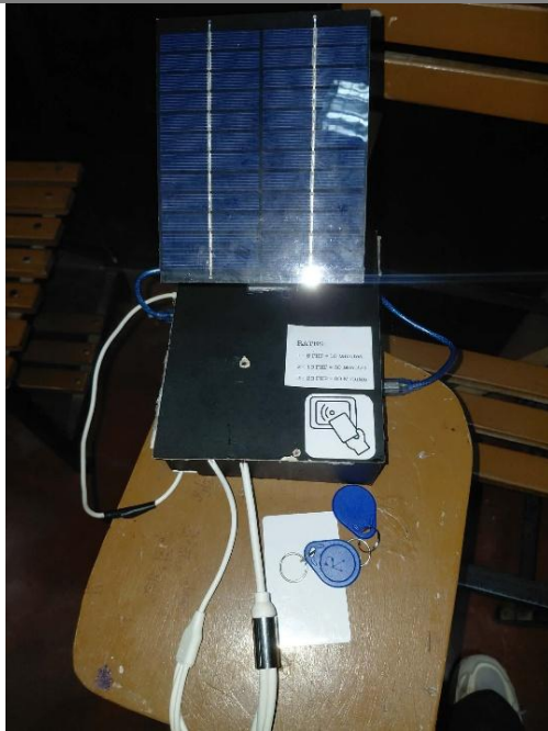
Figure 1. Completed RFID-Based Solar-Powered Portable Phone Charging Station Prototype Integrating the Arduino Uno R3, MFRC522 RFID Reader, HC-05 Bluetooth Module, Dual-channel Relay Module, Solar Panel, Power Banks, and Android Application Connectivity.
