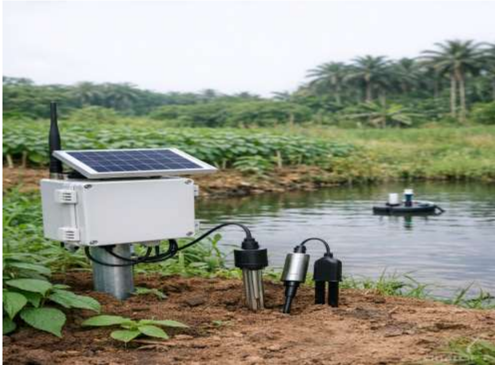
Figure 4.1 Prototype Low-Cost Wireless Sensor Network for Monitoring Soil and Water Parameters
