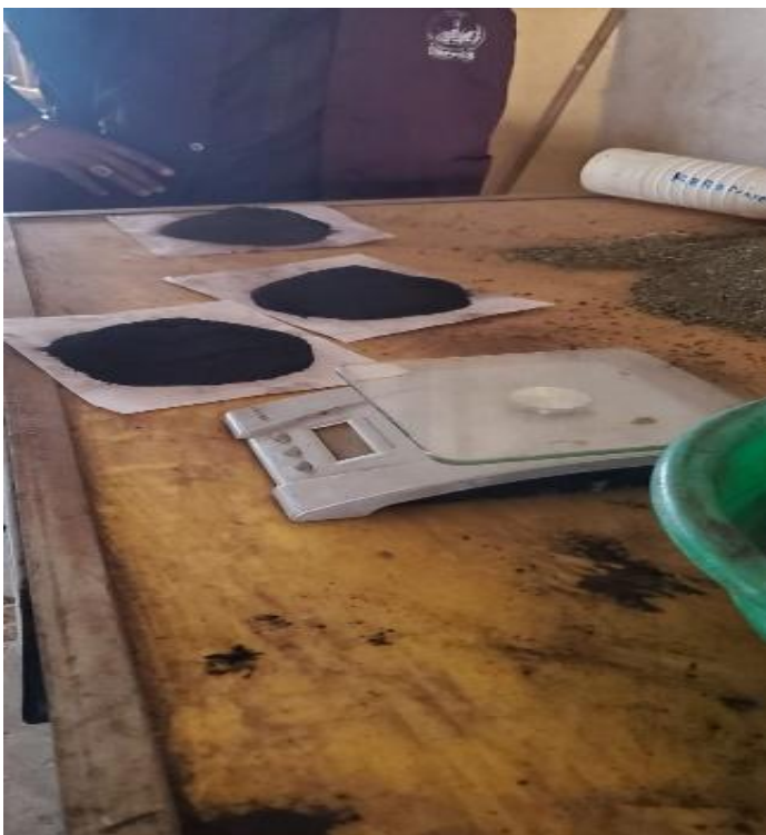
Plate 1. Dried Concentrates and Tailings Weighing Conducted at the Laboratory of the Department of Mineral & Petroleum Resources Engineering, Kaduna Polytechnic.
