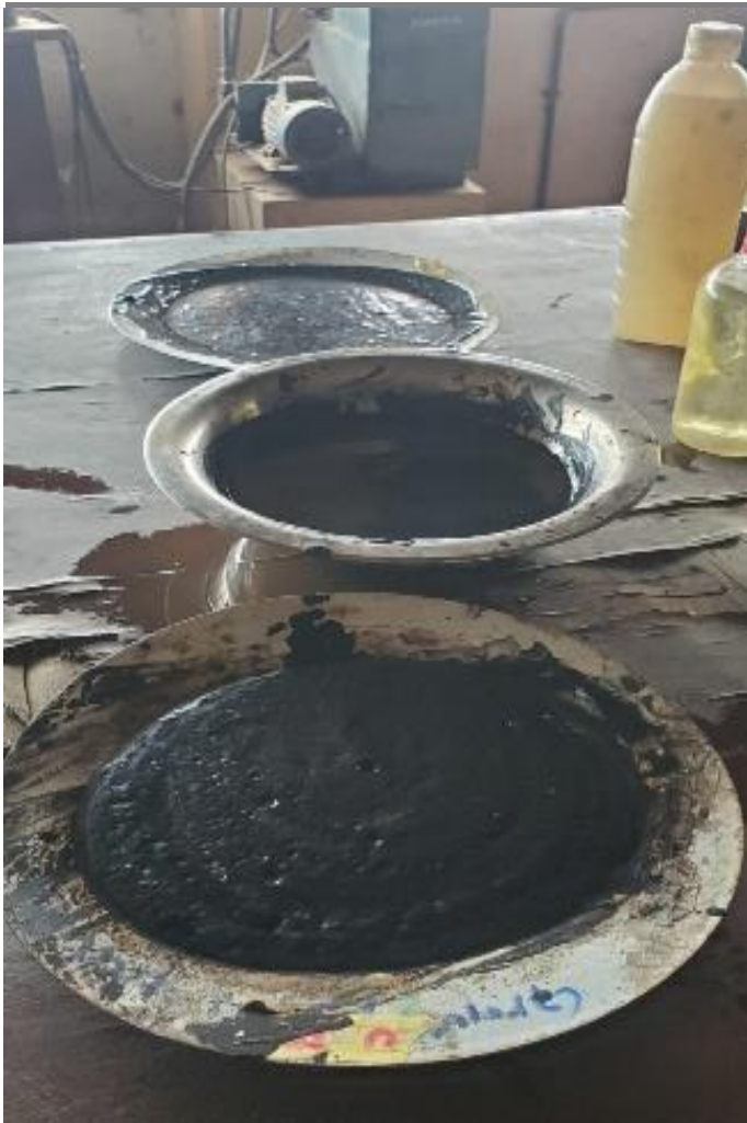
Plate 1. Wet Concentrates and Tailings of the sample after flotation Conducted at the Laboratory of the Department of Mineral & Petroleum Resources Engineering, Kaduna Polytechnic.
