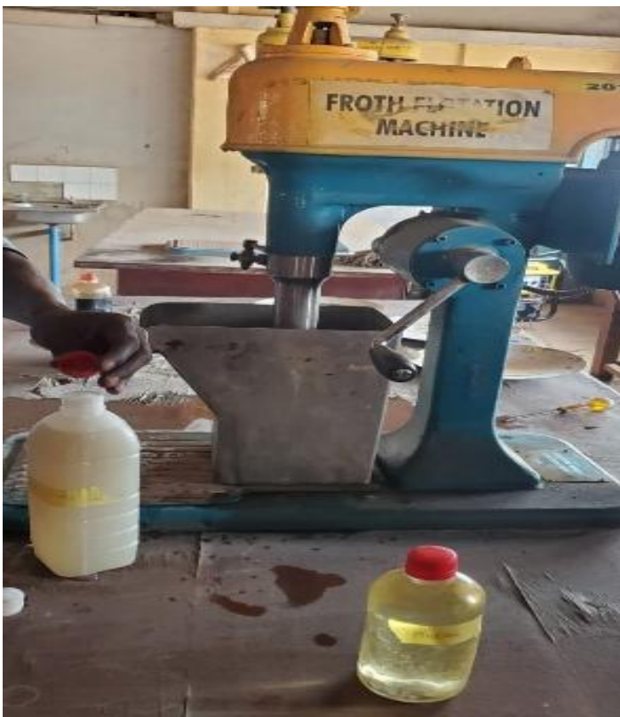
Plate 2. Flotation Procedure setup Conducted at the Laboratory of the Department of Mineral & Petroleum Resources Engineering, Kaduna Polytechnic.
