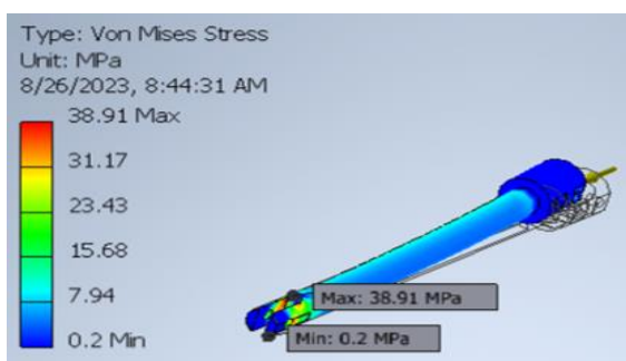
Fig. 2. Finite element stress analysis of the slotting ram shaft
