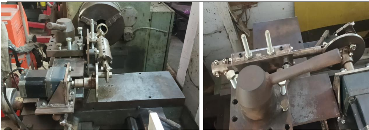
Fig. 4. Fabricated and assembled integrated slotting mechanism mounted on a conventional lathe.
