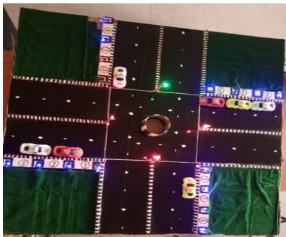
Figure 8: Testing the prototype for identifying and giving priority to road with highest traffic volume
