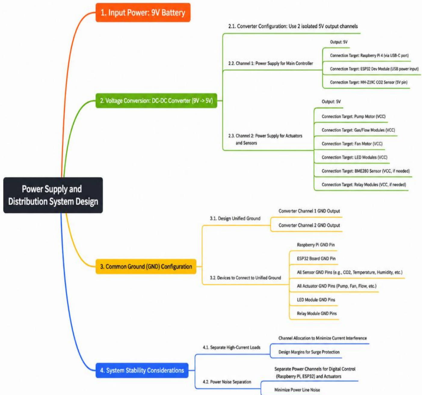
Figure 7. Separated power distribution and common ground design.
