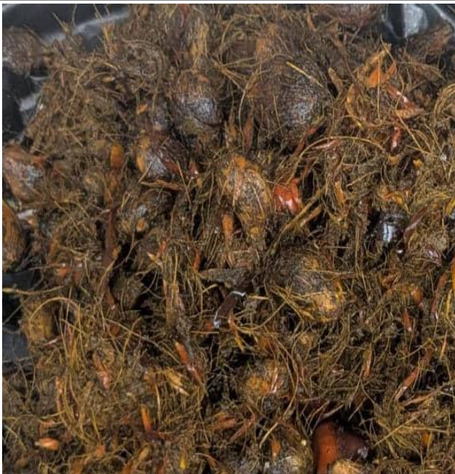
(c) Sample of digested palm fruits after being process in the digestion machine
