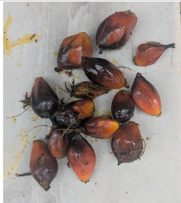
(d) Sample of undigested palm fruits after being processed in the digestion machine
