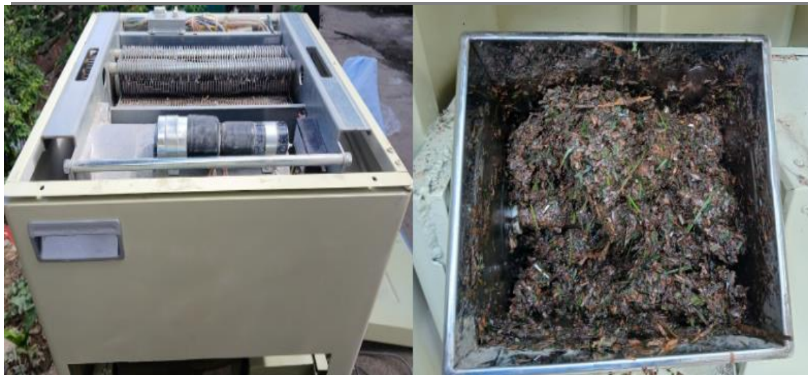
Fig.7 Shredded Organic Matter. The input materials used for composting were manually shredded using an organic material shredder. The shredded organic matter was standardized to a particle size of approximately 3 to 4 millimeters to ensure uniformity and increase the surface area available for microbial degradation (Resmi, G., & Vinod, V., 2022).
