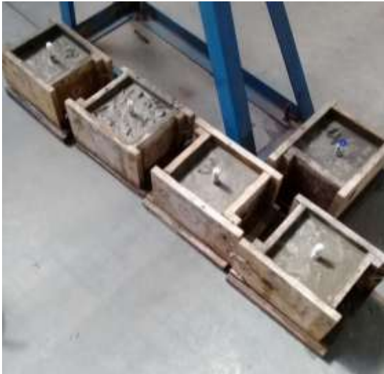
Fig (6) casting the concrete cubes.
