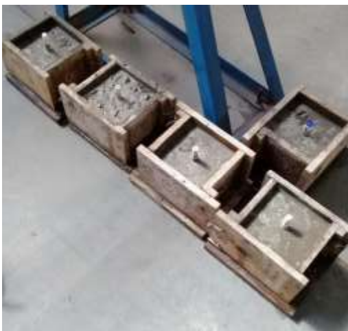
Fig (9 ) making the holes on the blocks.
