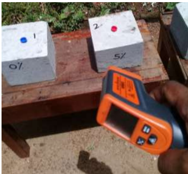
Fig (12 ) Temperature measuring the surface of the concrete blocks
