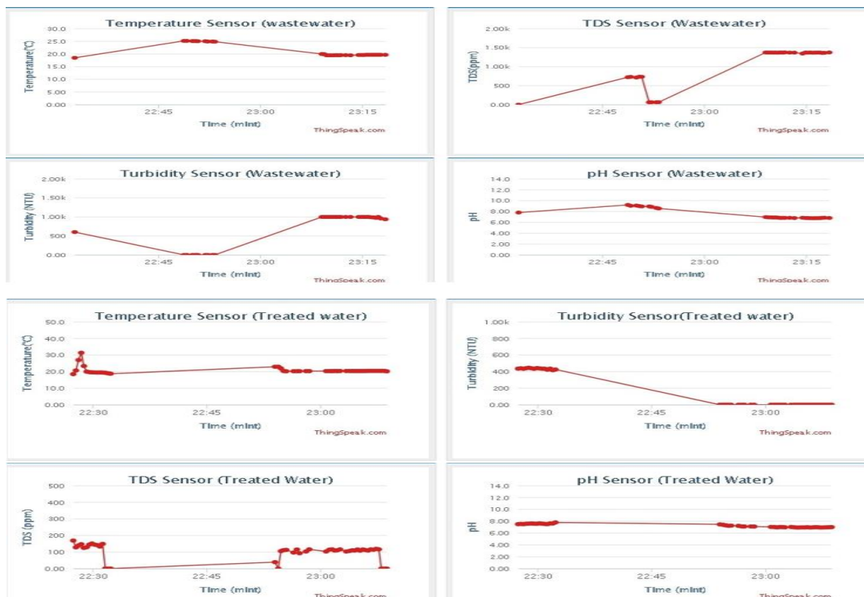
Figure 4. ThingSpeak IoT dashboard showing real-time sensor data
